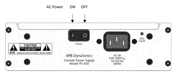
Turn on each power supply using the rocker switch on the PS panel.
